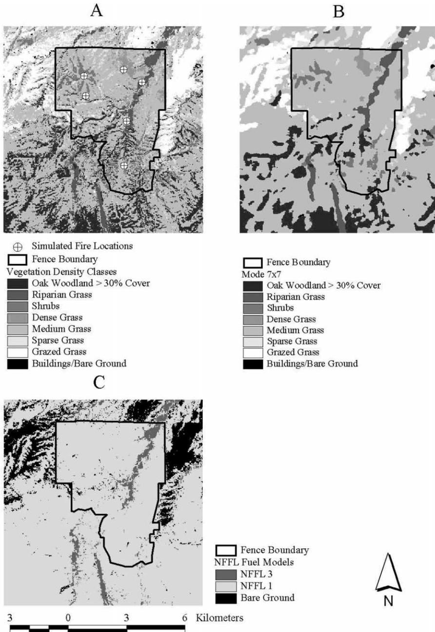
Fig. 3. Fuels maps: (a) high resolution custom fuels map based at 30 m mapping resolution derived from a Landsat TM image, August 25, 1996 (overlaid with random fire start locations used in the simulations); (b) low resolution custom fuels map at 210 m mapping resolution (30 m pixels) fuels map generated by degrading the high resolution custom map with a  $7 \times 7$  mode filter; (c) fuels map using NFFL fuel models at 30 m mapping resolution.
